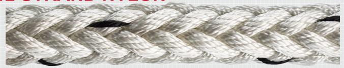
Traditional 12-Strand Nylon ropes are used in numerous applications. Nylon has high elongation and a higher tenacity than polyester. Torque balanced construction with firm round profile, is easily spliced, and used for general working lines, secondary mooring lines, mooring pendants, and slings and strops.
