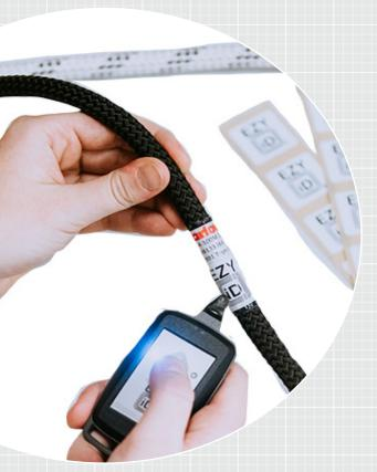
Using state of the art RFID technology, EZYiD uses the EZYiD Reader/Writer as a RFID key fob, capable of reading any EZYiD product and transmitting stored data with the push of a single button - empowering the EZYiD reader as a Human Interface Device (HID) which enables versatility across all software platforms.
